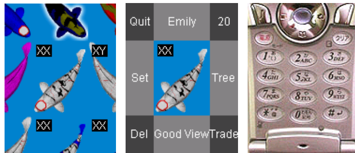
Fig. 2. Discrete panning with partial context (left), the KeyPadPie menu (middle), and the Mitsubishi Electric J-D05 J-Phone keypad (right).
