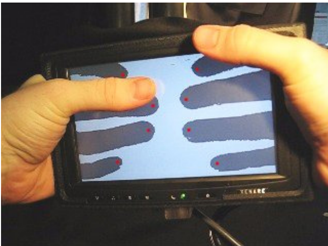
Figure 2. The LucidTouch prototype.
