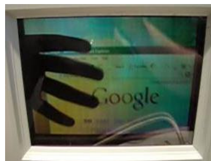
Figure 3. Our first LucidTouch mock-up created a physical see-through effect using a modified overhead-projector LCD. It's main drawback: lack of illumination led to occlusion when touching the screen.
