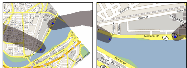
Figure 9. Our map browser application: the map rotates, translates, and scales to remain under the user's fingers.
